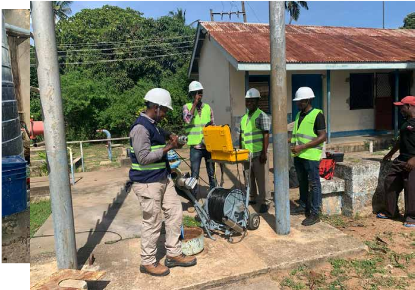
Borehole Camera inspection to offer quick and comparatively inexpensive way to inspect, investigate and verify the downhole conditions at depths not easily reachable by other means.
