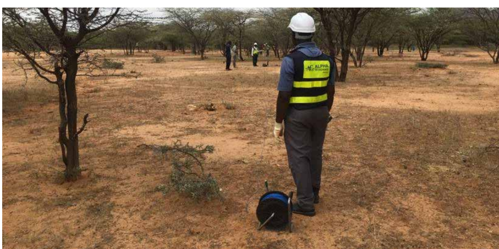
Borehole Camera inspection to offer quick and comparatively inexpensive way to inspect, investigate and verify the downhole conditions at depths not easily reachable by other means.
